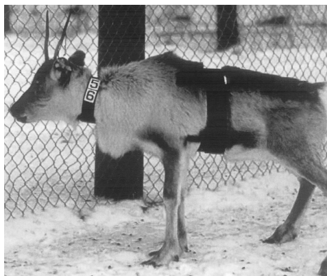
Figure 2. The wrist monitor was attached to the collar and the transmitter to the fur. An elastic band was used to secure the attachment of the transmitter. Photo by Harri Nurminen.
