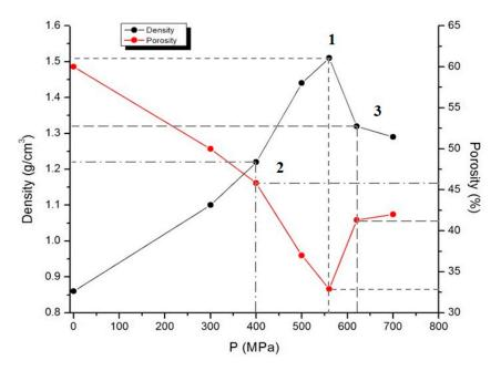
Figure 4. Density and porosity-pressure diagram for samples 1–3.
