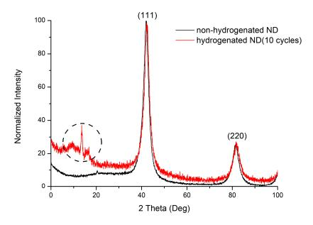
Figure 7. Diffraction pattern of non-hydrogenated and hydrogenated nanodiamonds.
