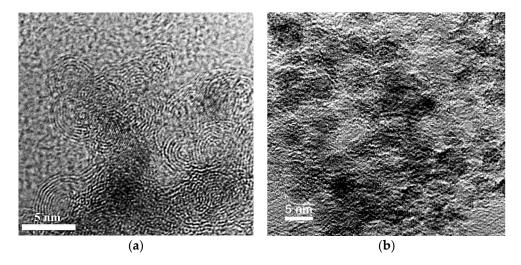
Figure 5. TEM images of the nanodiamonds material: (a) carbon onions; and (b) nanodiamonds.
