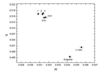
**Figure 11.** Dependence of the *S*-parameter on the *W*-parameter for non-hydrogenated and hydrogenated nanodiamond samples.
