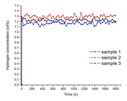
Figure 6. Hydrogen concentration in the samples 1–3 after the first cycle of sorption.
