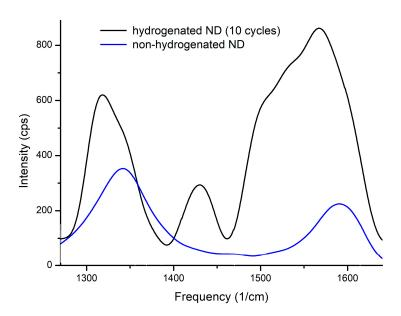
Figure 8. Raman spectroscopy of non-hydrogenated and hydrogenated nanodiamonds.
