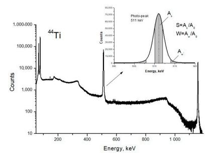
Figure 3. Energy spectrum of scintillator BaF<sub>2</sub> detector and line shape parameters of the photo-peak.
