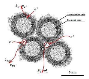
Figure 2. Model of delayed formation of positronium in nanodiamonds.
