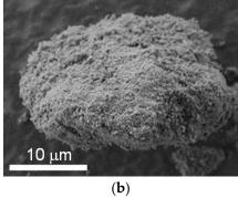
Figure 1. Transmission (a) and scanning (b) microscopy micrographs of nanodiamonds.
