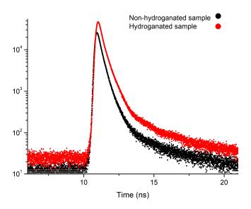
**Figure 9.** Positron annihilation lifetime spectra measured for non-hydrogenated and hydrogenated nanodiamond samples.
