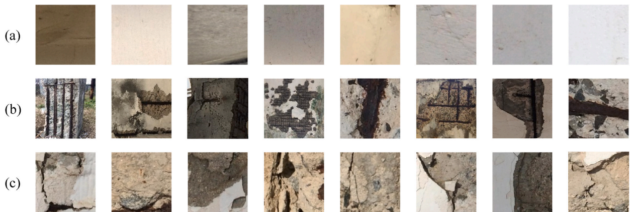
Fig. 2. Image dataset of undamaged and damaged RC: (a) Undamaged areas, (b) Exposed reinforcement, (c) Spalled concrete.
