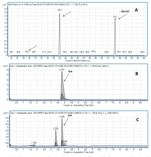
**Figure 2.** (**A**) Product ion mass spectra of protonated IAA (5.71  $\mu$ mol L<sup>-1</sup>) recorded by flow injection analysis. Ions selected for MRM are marked with arrows. (**B**,**C**) Example of MRM results obtained during LC-MS/MS analysis of the IAA standard solution (**B**,**C**) bacterial culture supernatant of strain HLA 1-7 after 144 h of culturing.
