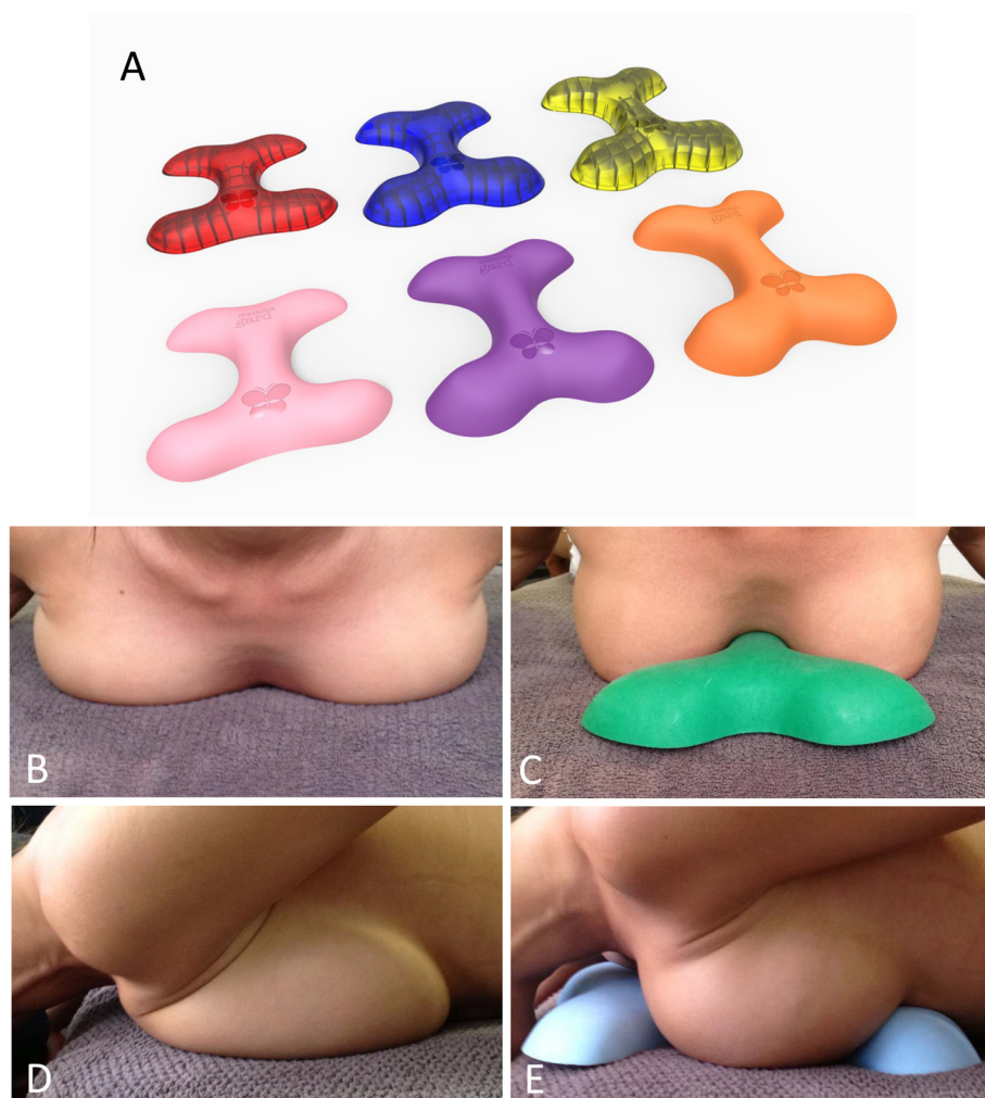
Figure 1 Orthosis in different sizes and densities, the transparent models illustrate the orthosis' ribbing for adjustment of firmness (A); Participant positioning on the orthosis in cephalic view (B), side view (C), lateral view without the orthosis (D) and with the orthosis (E).
