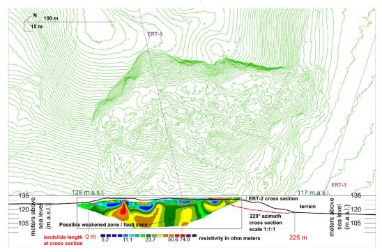
**Figure 11.** Hrvatska Kostajnica landslide cross section (perpendicular to movement) and interpreted ERT-2 data. At cross section area the length of the landslide is 225 m with slide surface at the depth of ~10 m. In the middle part of the cross section possible fault zone is present (marked with question mark). The contour line interval on the topographical map is 1 m.
