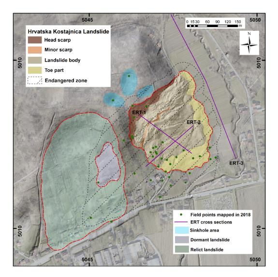
**Figure 8.** New Hrvatska Kostajnica Landslide Map with marked areas of active, dormant and relict landslide. Landslide areas are depicted with red dashed lines. On the map re-defined area of landslide(s) endangered zone is also marked (grey dashed polygon area).
