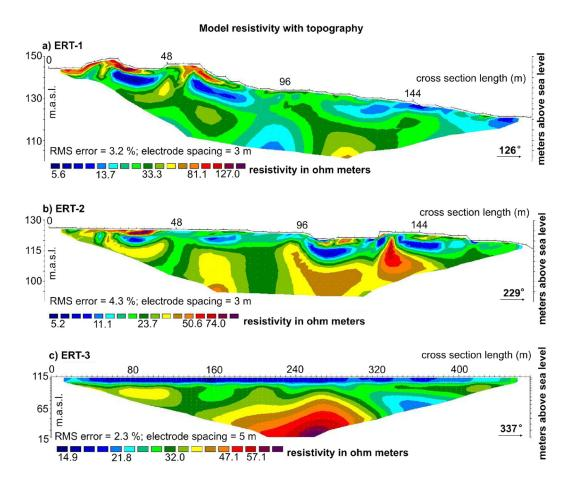
**Figure 9.** Electrical resistivity tomography results: (a) ERT-1 in the landslide body, cross section is oriented along the movement direction; (b) ERT-2 in the landslide body, cross section is oriented vertically on the movement direction; and (c) ERT-3 in the vicinity of the landslide, cross section is located in the "undisturbed soils". On the ERT-1 and ERT-2 highly deformed/disturbed near surface areas can be depicted while on ERT-3 paleo-relief can be interpreted.
