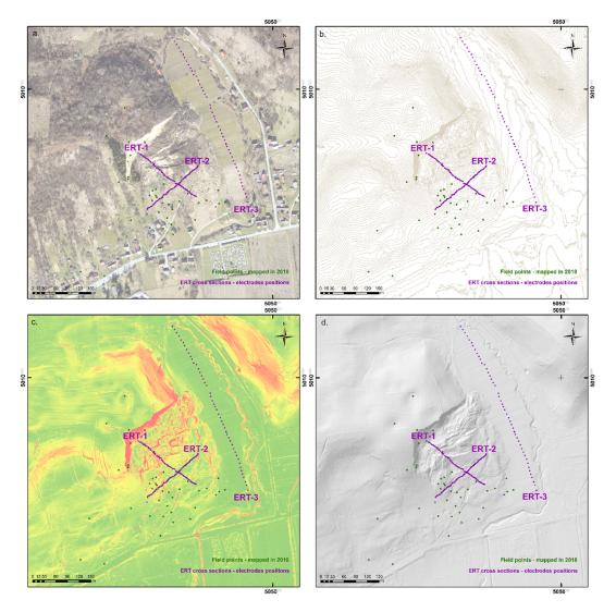
**Figure 7.** High resolution data from the Hrvatska Kostajnica area and landslide study area with mapped field points from 2018 and locations of ERT cross sections from 2020 and 2021: (a) detailed orthohpto from 2021; (b) 1 m contour lines based topography map; (c) detailed slope model; and (d) detailed terrain hillshade model.
