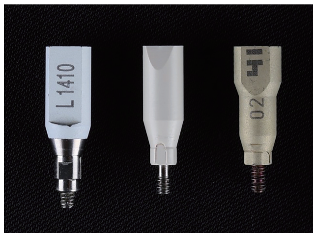
Fig. 1. From left to right, non-original, original and generic scan bodies with cylindrical geometry varying in features.
