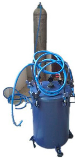
Figure 2. Apparatus of the accelerated carbonation test.
