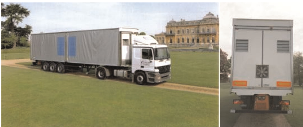
Figure 23: Mechanically ventilated vehicle that uses curtains and a fan in the tailboard for ventilation (Courtesy of Malcolm Mitchell)
