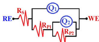
Figure 11. Equivalent circuit represents the best EIS data fit.
