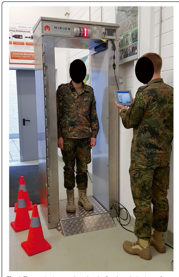
Fig. 1 The monitoring portal used at the Bundeswehr Institute of Radiobiology (CheckPoint: Gate™ FastTrack-Fibre™ Mobile) with technical specifications. Detection limits are given for different measurement modes and times [32]. Lead shielding 15 mm: cesium-137 [wait in (5 s): 1.35 kBq; walkthrough (0.57 s): 4.8 kBq], americium-241 [wait in (5 s): 29 kBq; walkthrough (0.57 s): 105 kBq]. Lead shielding 30 mm: cesium-137 [wait in (5 s): 1.25 kBq; walkthrough (0.57 s): 4.5 kBq], americium-241 [wait in (5 s): 28 kBq; walkthrough (0.57 s): 100 kBq]
