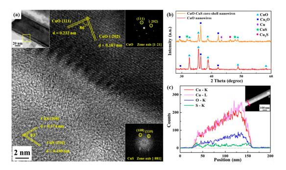
**Figure 3.** (**a**) TEM and HR-TEM images, (**b**) XRD analysis, as well as (**c**) line scanning profile and high angle annular dark field (HAADF) image of CuO-CuS core-shell nanowire(s).
