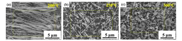
**Figure 2.** FE-SEM images of CuO nanowires under sulfurization process at different temperatures (**a**) 200 °C, (**b**) 250 °C, (**c**) 300 °C.
