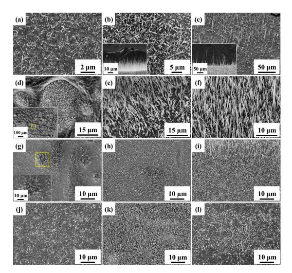
**Figure 1.** FE-SEM images of CuO nanowires grown at different temperatures (**a**) 350 °C, (**b**) 550 °C, (**c**) 800 °C, for different oxidation time (**d**) 0 h, (**e**) 1 h, (**f**) 2 h, with different ramping rates (**g**) extremely fast, (**h**) 8 °C/min, (**i**) 4 °C/min, and under different oxygen concentrations (**j**) 10%, (**k**) 50%, (**l**) 100%.
