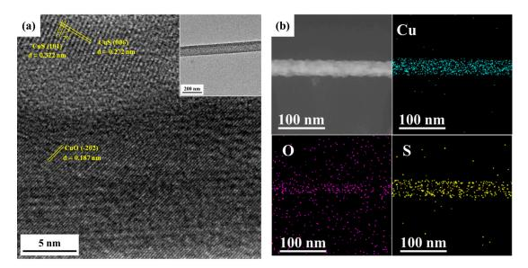
**Figure 7.** (a) TEM analysis and (b) EDS mapping of the CuO-CuS nanowire after 4 cycles of photocatalytic reactions
