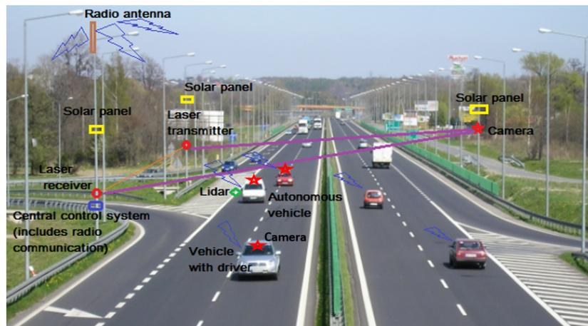
**Figure 14.** Proposal for a system to increase traffic safety in real traffic conditions.
