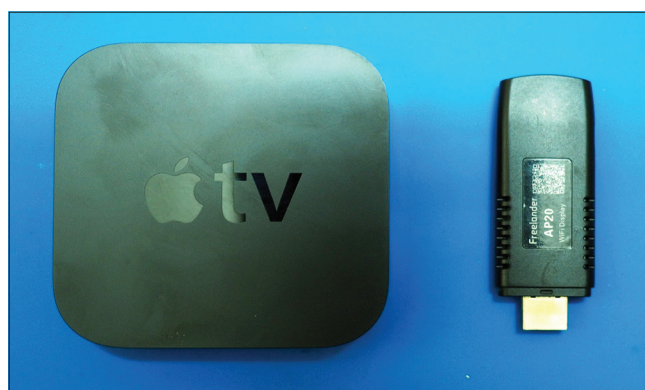
Figure 2: Apple TV and Miracast Screen Mirroring modules for use with iOS or Android devices, respectively
