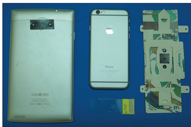
Figure 1: An android phone/tablet (phablet) – Chuwi VX1 with the magnetic strip connector affixed to the rear camera, an iPhone 6, the Foldscope and a demo slide (ground section/DE Junction)
