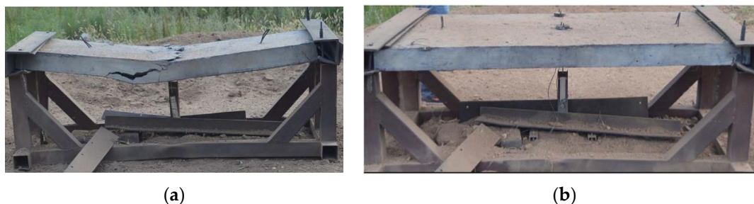
Figure 2. The detonation of (a) normal concrete; (b) PE-ECC [91].
