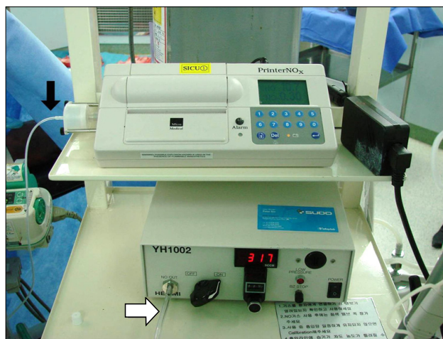
Fig. 3. The photograph shows a NO gas dosage machine (PrinterNOx, Micro Medical Ltd., England), NO gas supplying line (white arrow) and monitoring line (black arrow).
