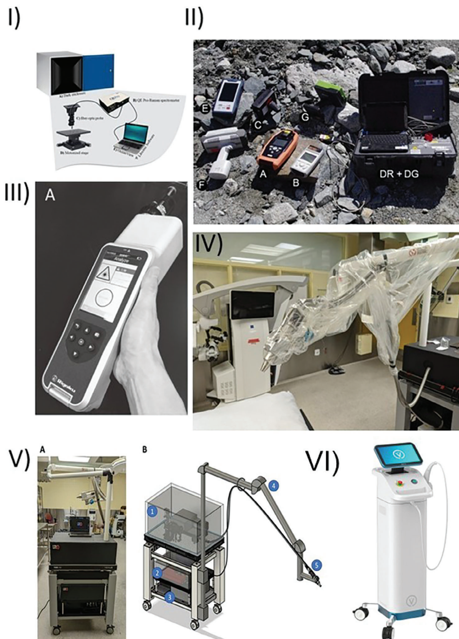
Figure 8. Portable Raman systems demonstrating variation in size, portability and style. I) Portable technology utilized to detect spoilage in food. [133] Copyright 2022, MDPI. II) Miniature Raman spectrometers used to beryl in a model study a) FirstDefender XL, b) FirstDefender RM, c) Inspector Raman, dr/dg: EzRaman-l, e) Bravo, f) FirstGuard, and g) RaPort as reviewed by Jehlička et al. [149] Copyright 2017, Wiley. III) Progency spectrometer employed for the detection of colorectal cancer adapted from. [150] Copyright 2019, J-Stage. IV) Illustration of an intra-operative system for the detection of skin cancer, showing a sterile drape secured with bands and sterile tape, while attached to a telescopic arm to aid in removability and insertion into surgical cavity (V). Both Va and Vb demonstrate overall device setup – used with permissions from. [141] Copyright 2023, RSC. VI) The most currently advanced commercial clinical Raman system by Vita Imaging Inc., used with explicit written permission, [148] copyright to the authors.
