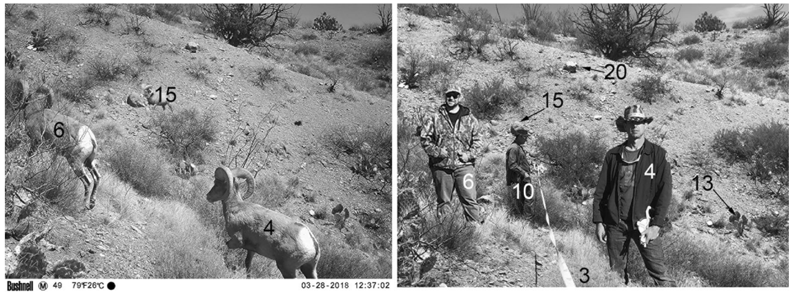
Figure 2. We measured the distances between desert bighorn sheep and the trail cameras imaging them, by printing out all of the sheep images, visiting the site, and positioning a human in the exact location that the sheep was imaged. We then used a range finder or metric tape to measure the distances. We supplemented these measurements by recording distances between the camera and several recognizable objects in the images (e.g. rocks, plants), to ensure accurate distance delineations for the sheep.
