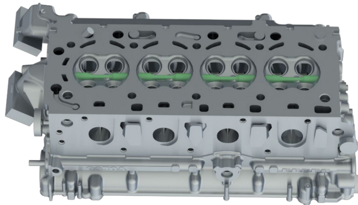
Figure 1. Illustration of test specimen extraction from the highly loaded valve bridge areas of a cylinder head.
