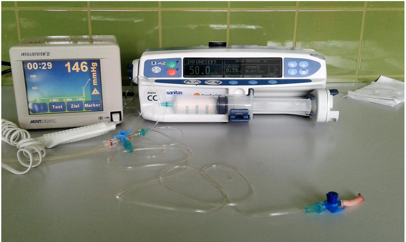
**Fig 10. Experimental setup.** The pressure transducer (Intellisystem II, Merit Medical) is on the left, the infusion pump (Alaris Care Fusion) is on the right, and the attached arterial segment is in the front.
