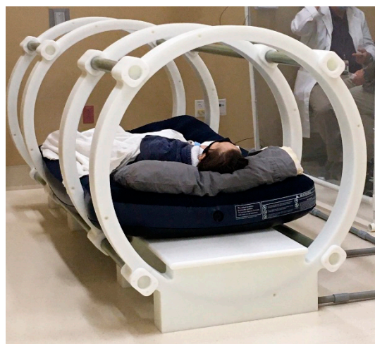
Figure 2. The photograph depicts the patient in the bore of the custom-built coaxial ring device used to deliver the uniform pulsed electric fields necessary for opening the VGSCs in TOL (The Phantom Laboratory, Salem, NY, USA).
