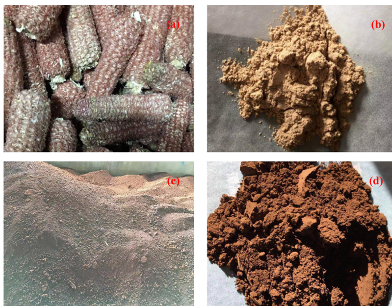
Figure 1. (a) Corn cob before crushing, (b) corn cob after being dried and crushed through a 150 \mu\text{m} sieve, (c) SHPS before crushing, and (d) SHPS after being dried and crushed through a 150 \mu\text{m} sieve.
