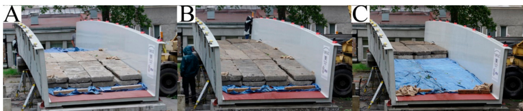
Figure 14. Loading sequence during the U3 test (from A to C).
