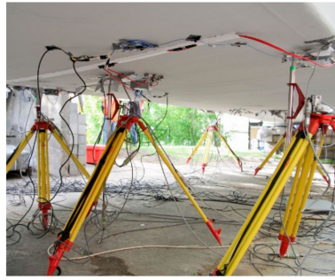
Figure 10. Inductive transducers used during measurements.
