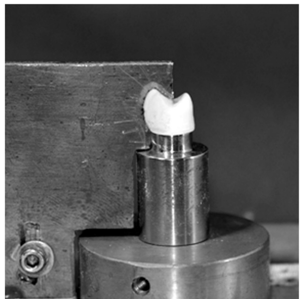
Figure 1. Illustration of the cutting template used to ensure a uniform 1 mm thickness of veneering material.
