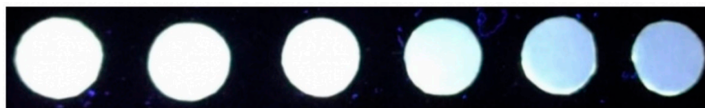
Figure 5. The photographs of MMN on test papers with different apparent pH solutions under a UV lamp (365 nm).
