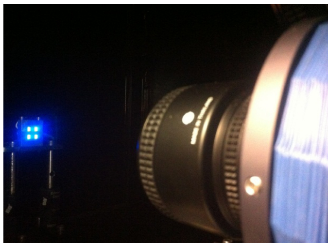
Fig. 6. High speed cameras (1/3 shown) are focused on the tiled array to detect fluorescence from the dyes. The application of masks over the matrix of fibres determines the focus of the cameras ensuring precise fluorophore variations.
