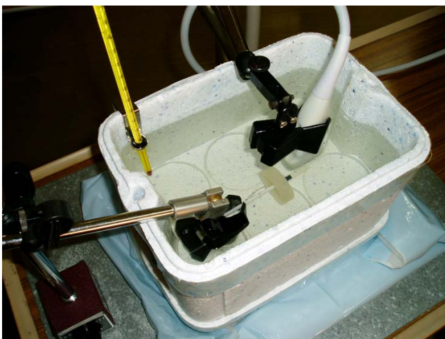
Figure 2 Scanning set-up for recording phantom images. Phantom and probe held in fixed position with stereotactic clamps in a water bath at approximately 37°C.
