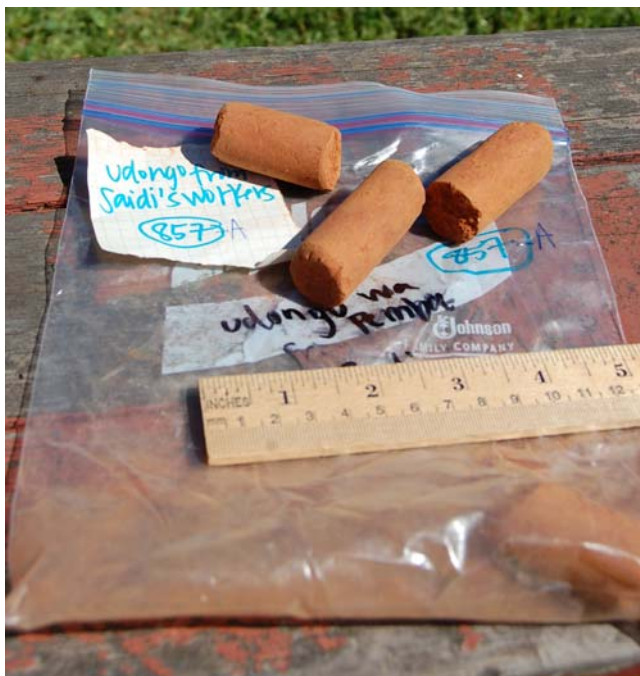
Figure 2. A close-up photograph of the sample in which the sample number is also visible is highly recommended. Ideally, a ruler should be included in the picture for scale. doi:10.1371/journal.pone.0003147.g002
