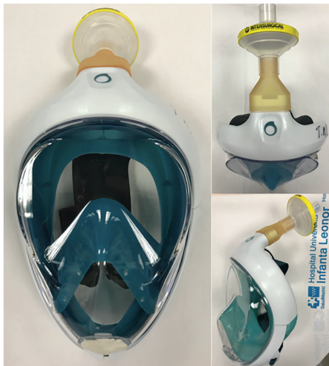
Figure 1. Adapted full-face snorkeling masks with an antiviral filter.
