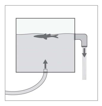
Figure 1. Chambers designed to assess the degradation of DNA from a silver carp carcass. Arrows indicate the direction of water flow.
