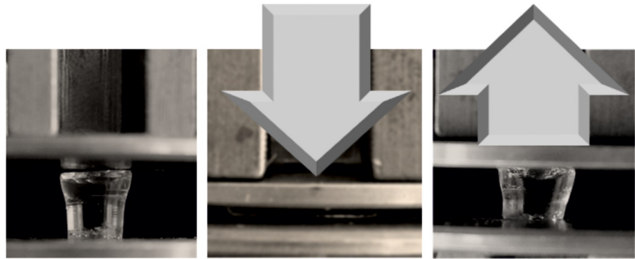
Fig 3. Compression and release of poly (TMA-VB) [22 ± 2 °C; M: 2 mol/L; MBAA 2 mol%].
