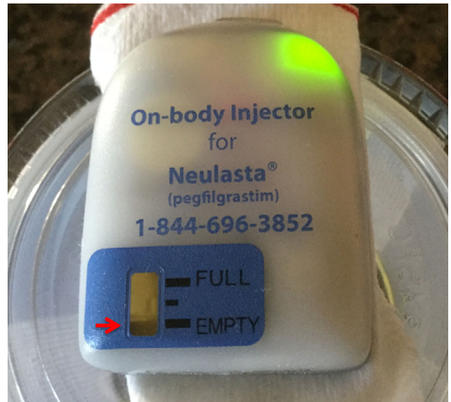
FIG. 4. Photograph of the device at the end of drug delivery after ten computed tomography scans with a cumulative dose of 230 mGy CTDIvol. As expected, the indicator read empty (arrow), and the status light flashed green.
