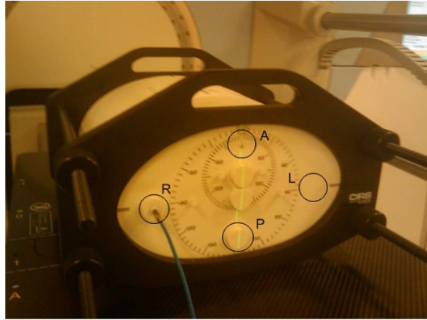
FIG. 1. Absolute dose for the 120 kV CBCT protocols involved the use of a CIRS body phantom. Doses were recorded at central and peripheral (A, P, R, L) locations.
