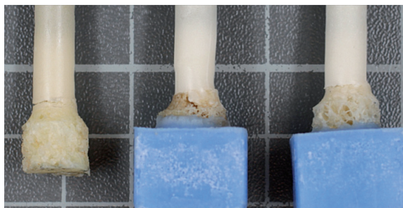
Figure 2. Representative examples of failure at the interface of the bone probes. On the left is an example of tensile failure. In the middle and on the right are examples of failure under torsion.
