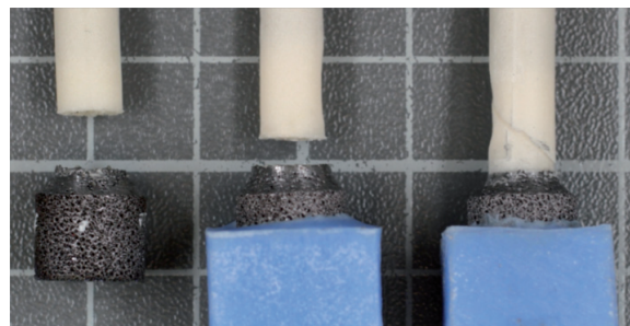
Figure 3. Representative examples of the failure modes of the porous metal-cement interface probes. On the left is an example of tensile failure. In the middle and on the right are examples of torsional failure.
