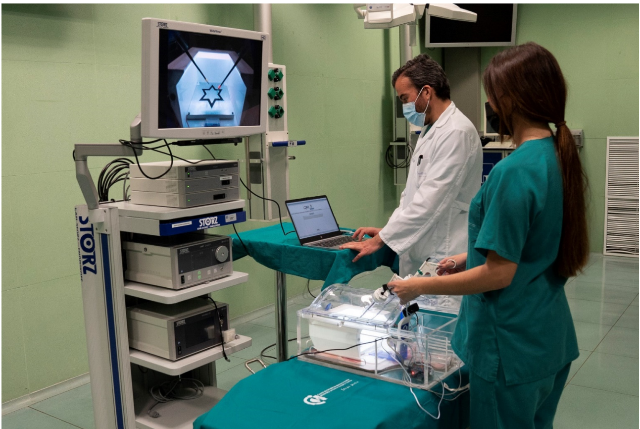
Figure 3. Setup of the experiment. ECG and GSR sensors are located inside the box trainer (red light). Eye tracker located immediately below the monitor showing the video feed captured by the camera inside the box trainer. The laptop is running the application gathering data. Research assistant is ready to start the second phase of the experiment, in which he will read mathematical questions out loud.
