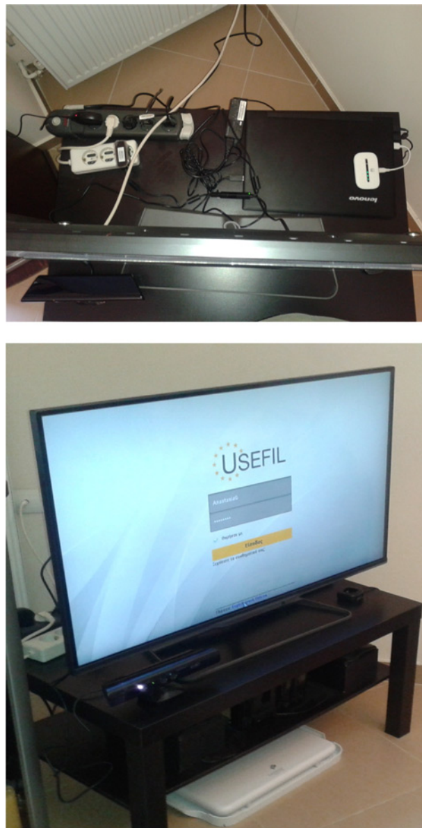
Fig. 1 Smart TV monitoring system setup top: laptop running Java monitoring app 24/7 plus connections; bottom: Philips smart TV
