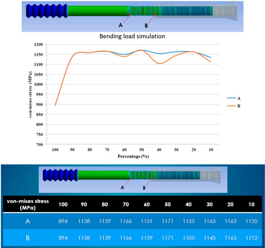
Figure 7. Stress at points A and B for different combinations in the bending load simulation. The length of engagement did not influence the stress distribution for combinations between 10% and 90%. The optimal combination is suggested to be greater than 90% to minimize the potential bending force. Higher von Mises stress, exceeding 1000 MPa, occurred at both Point A and Point B when the engagement length was less than 90%.
