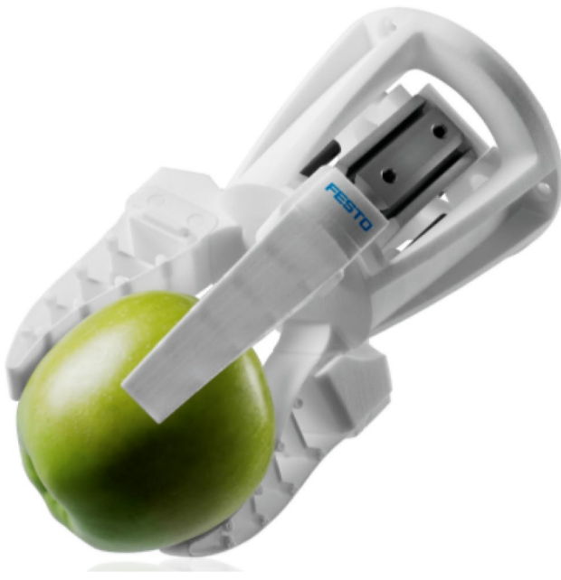
Fig. 3 Mechanical gripper with passive shape-adaptive elements [12]
