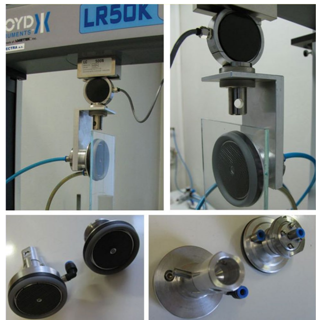
Fig. 31 Functional samples of designed gripping elements
