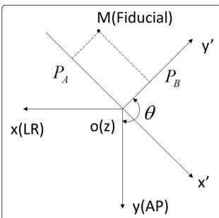
Fig. 3 Diagram showing projection and coordinate system rotation. The fiducial marker is at M;  $P_A$  and  $P_B$  are the two projection points
