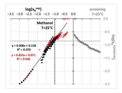
**Figure 2.** Results of benzamide solubility measurements and computations. All experimental points marked as black circles were taken from the literature while new measurements are presented as red plusses. Computed solubility values are presented in gray color. Dashed lines stand for best solubility values estimated so far at room temperature.
