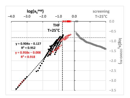
**Figure 5.** Results of salicylamide solubility measurements and computations. Notation is the same as in Figure 2.
