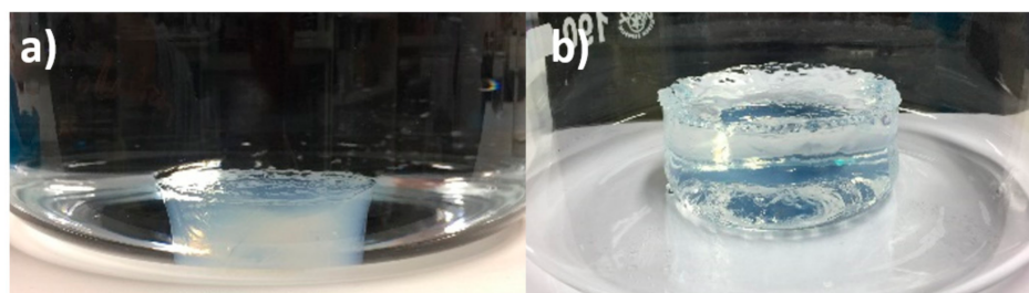
Figure 7. (a) Initial swelling of PAA1.5 hydrogel in de-ionized water (diameter: 64 mm, thickness: 22 mm); (b) swelling of PAA1.5 hydrogel for 8 days in 1.2 mol/L urea to reduce hydrogen bonding (diameter: 86 mm, thickness: 33 mm).
