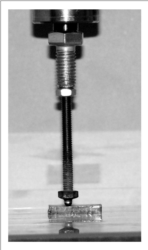
Figure 3. Spherical steel indenter, 3.2 mm in diameter, mounted on a material testing system (MTS Synergie 100, MTS Systems Corporation, Eden Prairie, MN), indenting a 3-mm-thick PAMPS/PDMAAm hydrogel specimen. This configuration was used for the nutrition (N)-related slow sinusoidal microindentation (SSMI) tests.
