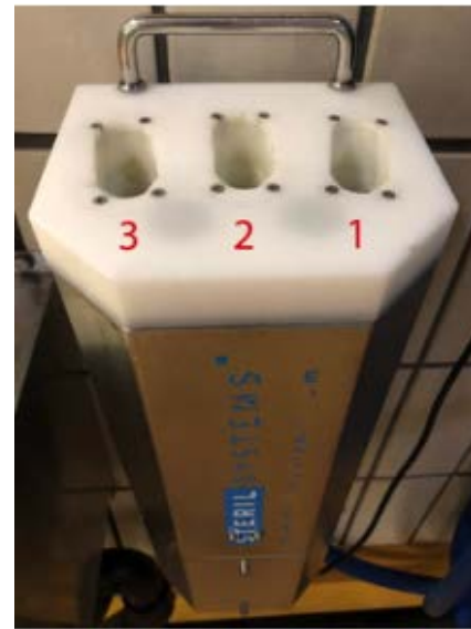
Figure 1. ME3-S device (Sterilsystems GmbH, Mauterndorf, Austria) for UV-C decontamination of knives with the different blade insertion sites (positions 1 to 3).
