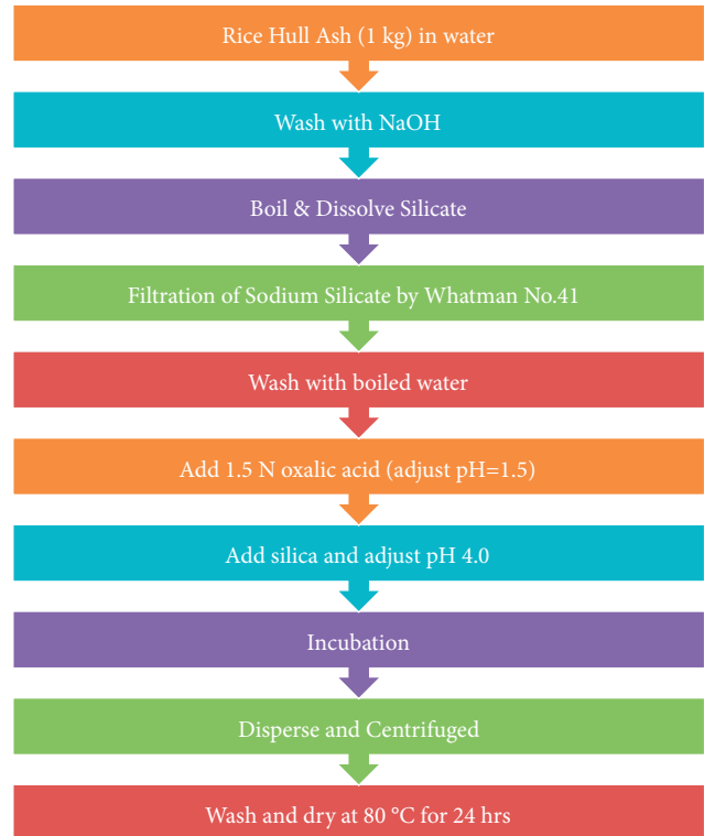
FIGURE 1: Flow diagram for extraction of silica from RHA.
