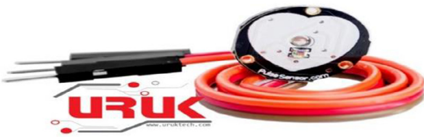
Fig. 7. Heart Rate (Pulse) Sensor for Microcontroller open source hardware development sensor.
