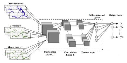
Figure 6. Example of a CNN computational model for inertial signal classification.
