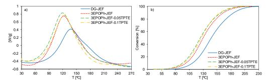
**Figure 4.** (a) Differential scanning calorimetry (DSC) thermograms corresponding to the dynamic curing at 10 °C/min of the formulations studied. (b) Conversion as a function of temperature of the formulations studied.
