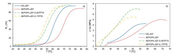
**Figure 7.** (a) Shape-recovery ratio as a function of temperature during the recovery stage under free conditions of all formulations. (b) Recovery stress generation as a function of temperature during the recovery stage under constrained conditions of all formulations.
