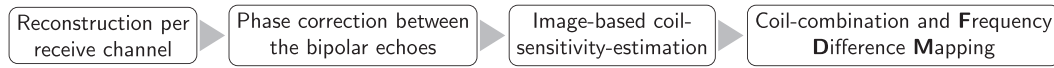
Fig. 1. Schematic representation of the processing pipeline. FDM allowed removal of the RF-related phase offsets and linear effect of large-length-scale field perturbations, without perturbing the local non-mono-exponential WM signal.
