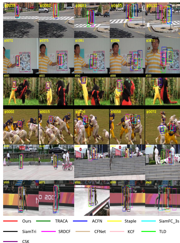
Figure 10. Quantitative tracking results of our tracker with other 10 trackers on OTB dataset. The video sequences are Couple, Doll, DragonBaby, Football1, Girl2 and Skating2_1 from top to bottom. The bottom illustration shows the colors for all trackers.
