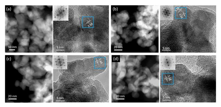
**Figure 1.** STEM and HRTEM images with corresponding Fast Fourier Transforms (FFT) of all studied catalysts: (a) Reference, (b) TiWet, (c) ZnALD and (d) ZnWet. In HRTEM images, interplanar spacings measured from FFT are provided (~3.3 Å (110), ~2.6 Å (101), family of planes of the SnO<sub>2</sub> structure).
