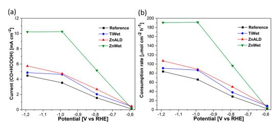
Figure 8. (a) CO<sub>2</sub>RR partial current density and (b) CO<sub>2</sub> consumption rate for all studied electrodes.
