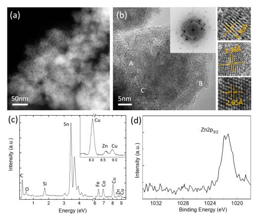
**Figure 7.** Characterization of tested ZnWet catalyst: (a) STEM image, (b) HRTEM images with corresponding FFT. Higher magnification images of A, B and C particles are also shown, and in these interplanar spacings calculated from FFT are provided ( $\sim$ 3.3 Å (110),  $\sim$ 2.6 Å (101) family of planes of the SnO<sub>2</sub> structure); (c) EDX and (d) XPS.
