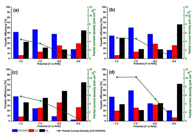
**Figure 6.** Faradic efficiencies for CO, HCOOH and H<sub>2</sub> formation and partial current density for electrodes: (a) Reference, (b) TiWet, (c) ZnALD and (d) ZnWet.
